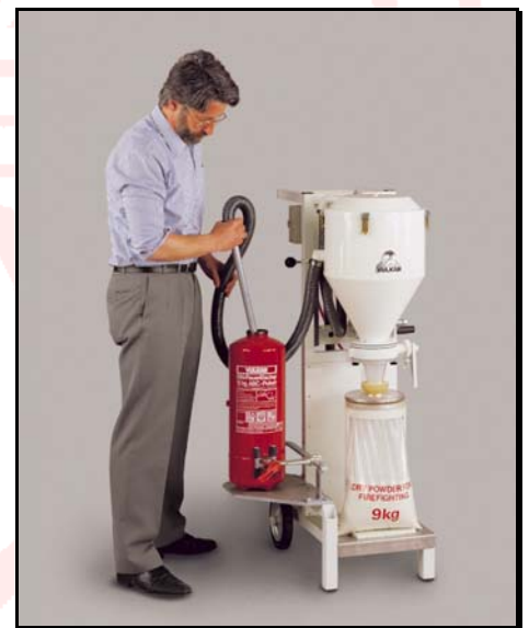
Discharge of old powder and filling in to plastic bags
