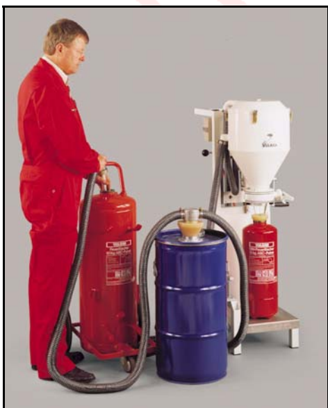
Emptying of wheeled extinguishers with storage drum and preliminary separator VA230
