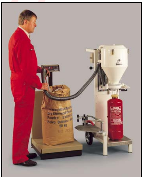
New filling of extinguishers place the powder storing container or storing sack on to the balance , and suction the required quantity of powder by means of the suction pipe into the extinguisher to be filled.
