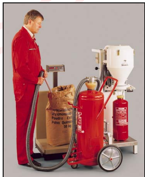
New filling of wheeled extinguishers with preliminary separator VA230
