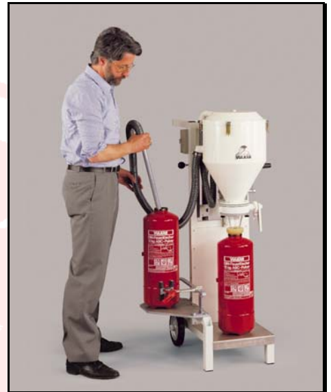
Refilling from one extinguisher to another
